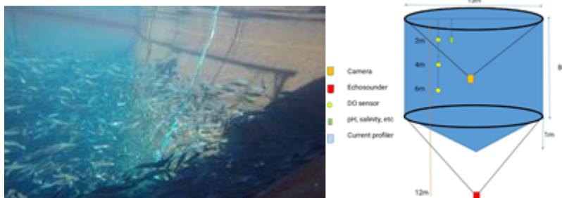
Figure 6: Setup of the environmental sensors at the pilot scale farm.
