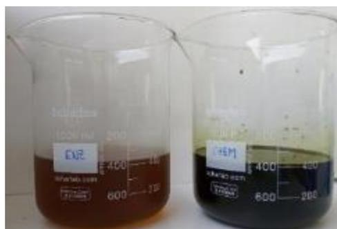
Figure 34 Medium ingredients obtained from insoluble matter *Nannochloropsis*. Left: ING insoluble Nanno – Enzymatic (process 3); Right: ING insoluble Nanno – Chemical (process 4)
