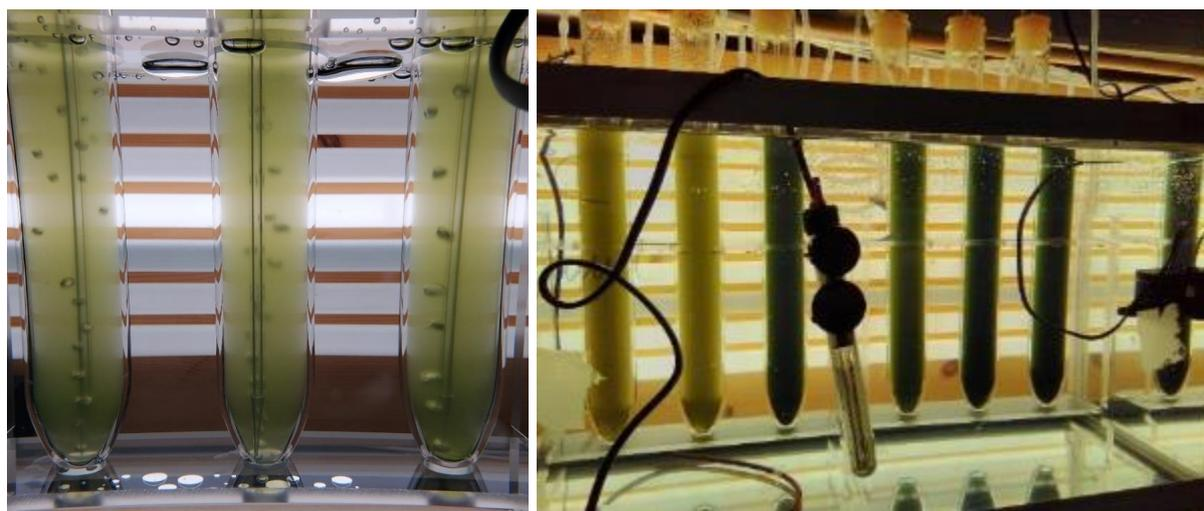
Figure 3 Bubble-column photobioreactors used for testing dirty water as nutrient source for microalgae growth (*C. vulgaris*).
