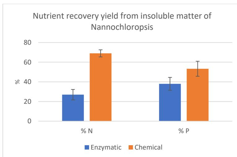
Figure 35 Nutrient recovery yield obtained from insoluble matter of *Nannochloropsis* by applying ultrasound pre-treatment followed by enzymatic hydrolysis (Process 3) and chemical hydrolysis (Process 4) at lab scale. Results expressed as percentage. Bar graph illustrating the mean and standard deviation (error bars) with n=3.
