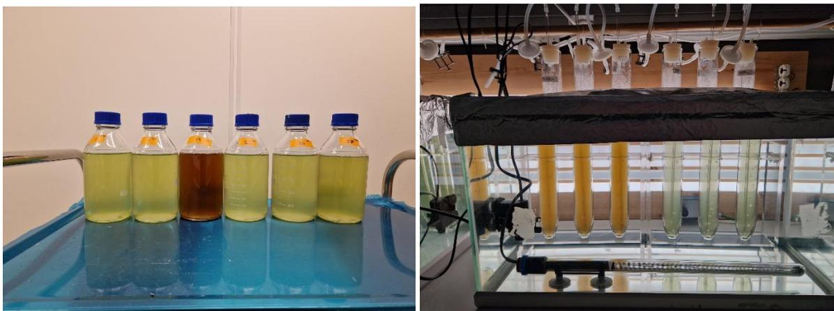
Figure 30 Left: Inoculum (*C. vulgaris*) on various waste streams (third bottle from left is on spent medium tested here, the other bottles contain wastewater from fish-farming (described in Chapter 3). Right: after inoculating in the bubble columns. The left three tubes are *C. vulgaris* on spent medium. The right three tubes are *C. vulgaris* on wastewater from fish-farming.
