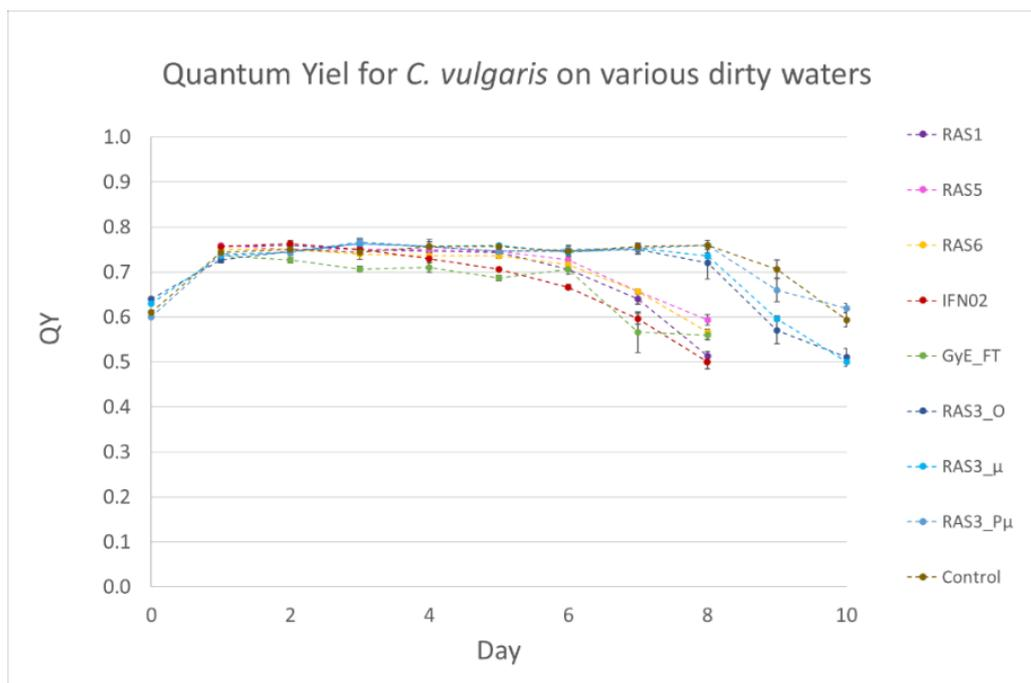
Figure 5 Quantum yield for *C. vulgaris* during growth on the various waste streams, and a control medium (BBM) in lab-scale bubble column photobioreactors.
