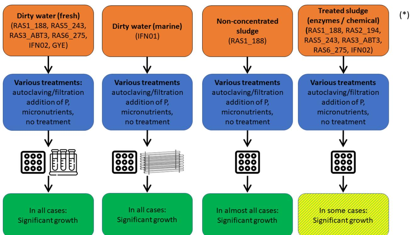
Figure 9 Overview of performance of microalgae growth (*C. vulgaris* or *N. gaditana*) on the various waste streams from fish-farming. (\*) Nutrients recovered from sludge as Medium Ingredient (MI) by applying enzymatic and chemical treatments.
