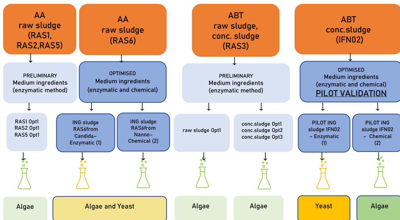
Figure 24 Summary of the medium ingredients (MI) obtained by LEITAT and delivered to NORCE for testing microalgae and yeast growth. In dark colour, the optimised medium ingredients. Conc.sludge from ABT: concentrated sludge using 60 micron filter, 15-20% dry matter. Sludge from AA: sludge from faeces collector, 0.5-4.3% dry matter
