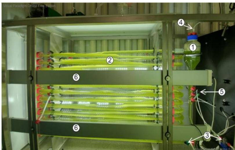
Figure 7 Photobioreactor used to test the dirty water from IFN\_01\_LC (Barramundi, seawater) for the production of *N. gaditana*. Explanation of points: 1. Main access point, 2. Tubular glass helix, 3. Aeration inlet and humidifier, 4. Deaeration, 5. pH-meter and thermometer, 6. Integrated LED-light panels.
