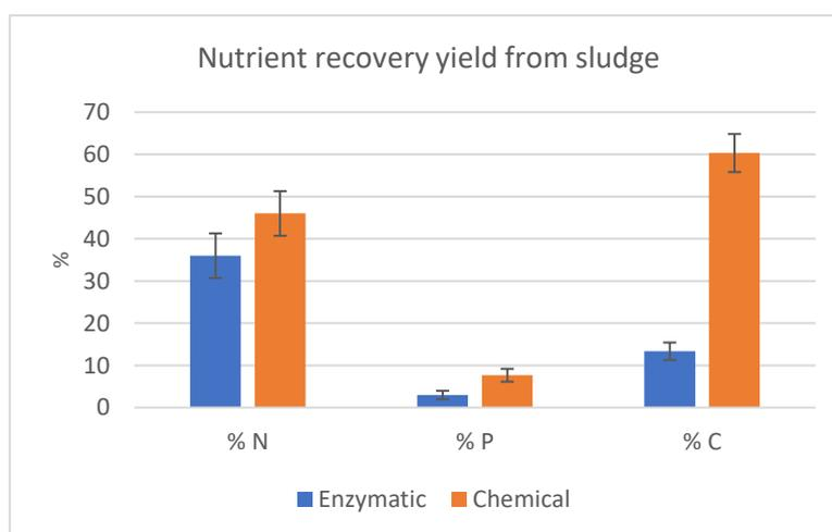
Figure 27 Nutrient recovery yield obtained from concentrated sludge IFN02\_RT by applying ultrasound pre-treatment followed by enzymatic hydrolysis (Process 1) and chemical hydrolysis (Process 2) at pilot scale (pilot validation). Results expressed as percentage. Bar graph illustrating the mean and standard deviation (error bars) with n=3.
