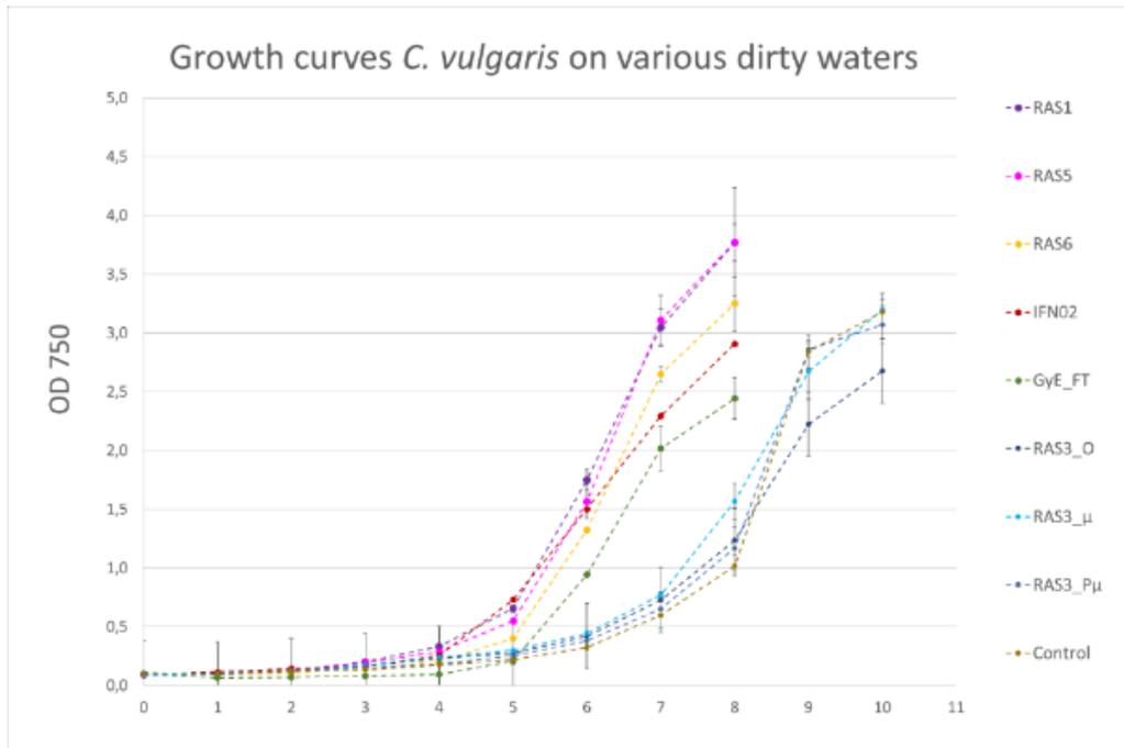
Figure 4 Growth curves of *C. vulgaris* on the various waste streams and a control medium (BBM) in lab-scale bubble column photobioreactors.
