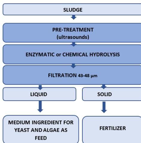
Figure 28 Sludge bioconversion process into nutrients (medium ingredients) at lab scale by applying ultrasound pre-treatment followed by enzymatic hydrolysis or chemical hydrolysis from raw sludge RAS6\_275, fish trial with rainbow trout and optimised new feeds
