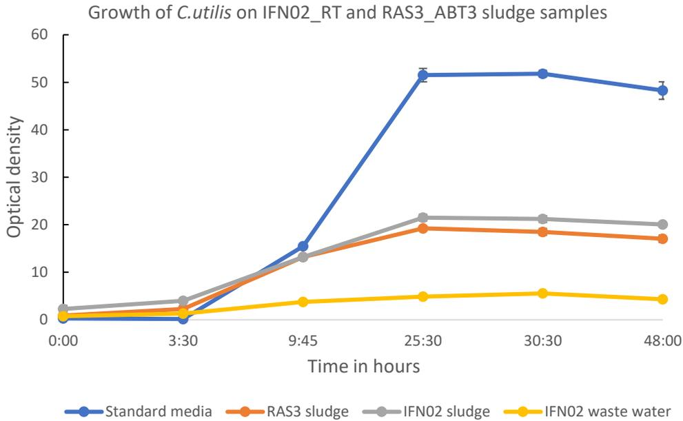
Figure 15 Growth of *C. utilis* on concentrate IFN02\_RT and RAS3\_ABT3 sludge without centrifugation step to remove the insoluble matter
