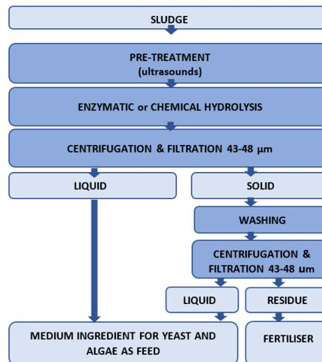
Figure 25 Optimised sludge bioconversion process into nutrients (medium ingredients) at pilot scale by applying ultrasound pre-treatment followed by enzymatic hydrolysis or chemical hydrolysis from concentrated sludge IFN02\_RT, fish trial with rainbow trout and conventional feed.
