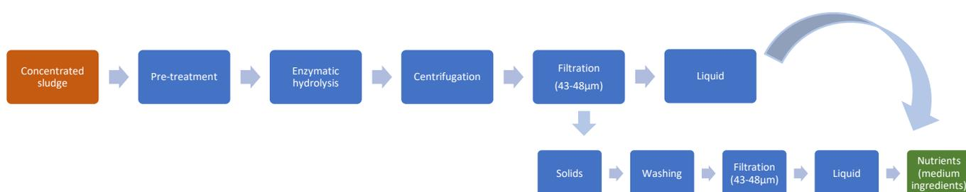
Figure 21 General diagram of sludge bioconversion process into nutrients (medium ingredients)
