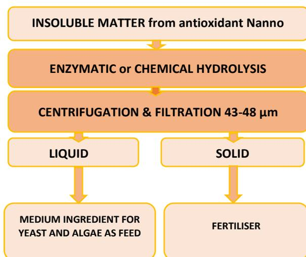
Figure 33 Optimised sludge bioconversion process into nutrients (medium ingredients) at lab scale by applying enzymatic hydrolysis or chemical hydrolysis from the insoluble matter from *Nannochloropsis gaditana*.
